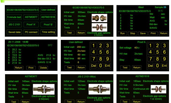
**KPM-OBD** is having Automatic Pre-programmed Test Sequences as per latest IEC/ ASTM . It is also capable of programming a customer defined test sequence .
