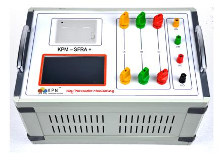
Sweep Frequency Response Analysis Test or in short SFRA Test can detect efficiently, displacement of transformer core, deformation and displacement of winding, faulty core grounds, collapse of partial winding, broken or loosen clamp connections, short circuited turns, open winding conditions etc.
