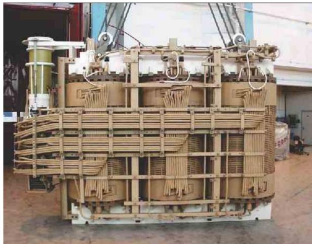
Any Movement inside Transformer changes the RLC equivalent which is Identified by KPM-SFRA+
