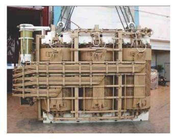
Any Movement inside Transformer changes the RLC equivalent which is Identified by KPM-SFRA01
