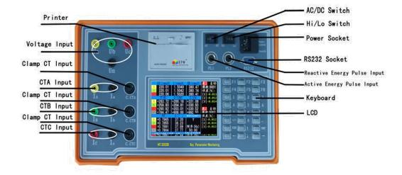
The calibrator is having a ABS plastic case, LCD display window and operation keys are located on the front of the calibrator, while power module is installed on the rear of it. There are 16 ports on the top of this calibrator:
