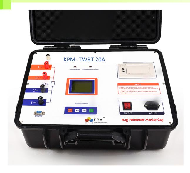
Winding resistance measurement of the Power Transformer is one of the critical test which ensures the healthiness of the transformer .
